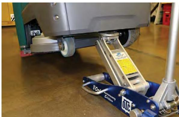
5. Place a jack stand underneath the other jack point and lower the machine onto the jack stand so both the jack stand and floor jack are supporting the weight of the machine.
