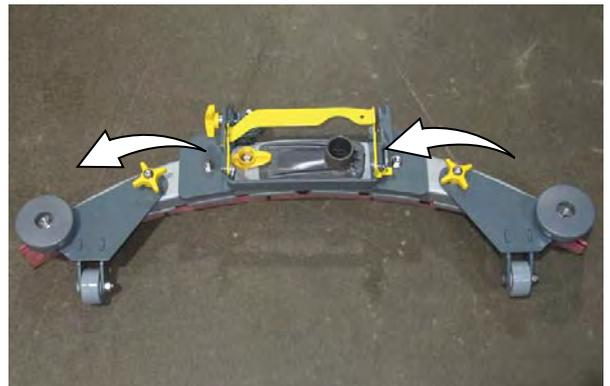
6. Remove worn blade(s) from the blade retainer.
