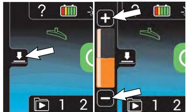
*NOTE: If brush pressure is set too high for scrubbing conditions, the brush pressure setting will automatically reduce to a lower setting and begin flashing. When flashing, reduce brush pressure to prevent brush motor overload.*
