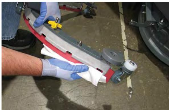
4. Clean scrub head skirt. Check for wear and damage. Replace if worn or damaged.
