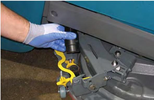
4. Squeeze the squeegee retainer lever and remove the squeegee assembly from the machine.
