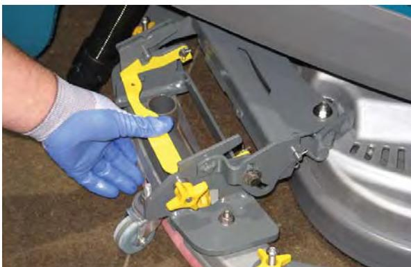
5. Fully loosen the two outside knobs on squeegee assembly. This will separate the spring loaded blade retainer from squeegee frame.
