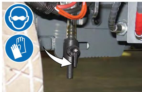
3. Close the battery compartment drain valve after all liquid has drained from the battery compartment.
