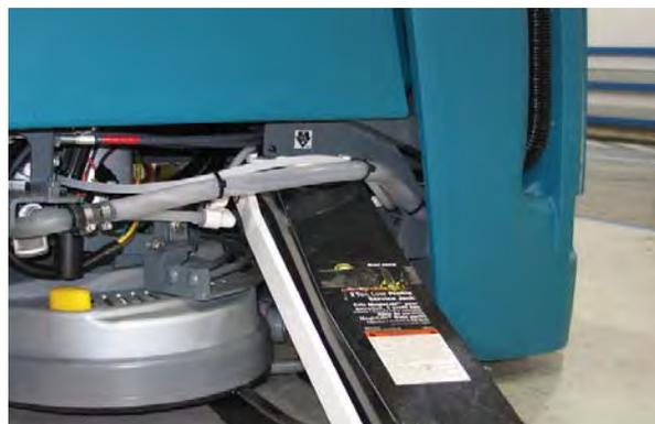
5. Use a floor jack to raise machine from the floor.
