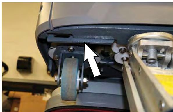
6. When finished with maintenance, use floor jack to raise machine from jack stand, remove the jack stand from under the machine, and lower the machine to the floor.
