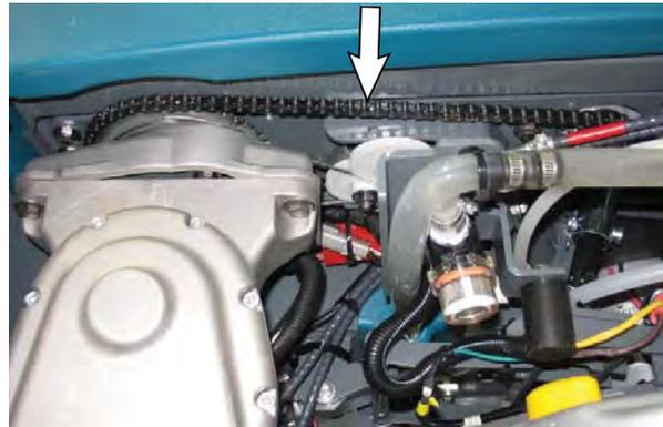
3. Check the steering cable for damage or wear. Use tension gauge to check steering cable tension.
