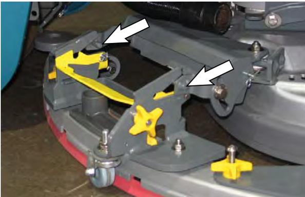
4. Slide the squeegee assembly onto the squeegee carriage until both squeegee carriage pins are secured in the bracket.
