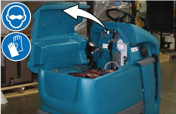
2. Carefully install the batteries into the battery compartment tray and arrange the battery posts as shown.
