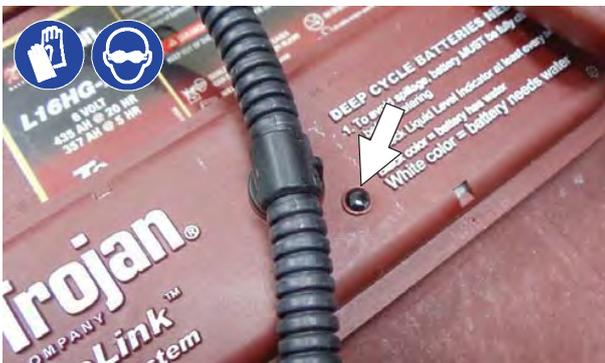
3. Locate the battery fill hose coupler inside the battery compartment. Remove the dust cap and connect the hand pump hose.
