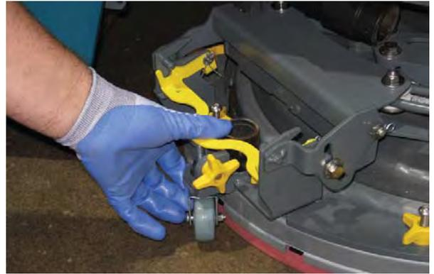
5. Fully loosen the four knobs on squeegee assembly. This will separate the spring loaded blade retainer from squeegee frame.
