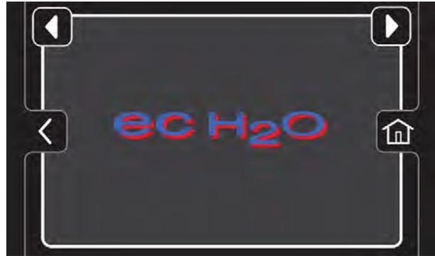
**Yellow ec-H2O Fault Screen** - Machine detected an ec-H2O system water or plumbing fault.
