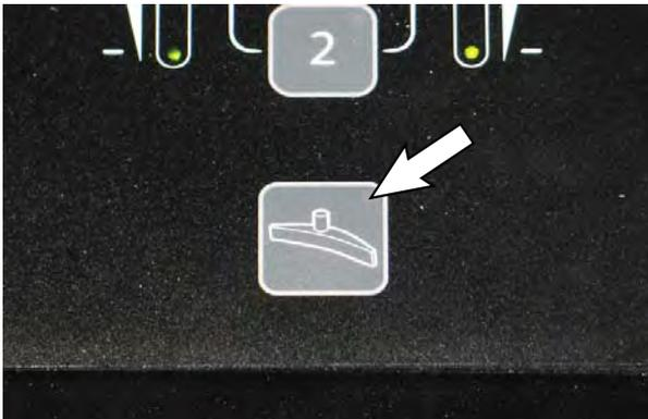
**Machines equipped with Pro-Panel:** Press the 1-Step button and then the vacuum fan button. The vacuum fan button will no longer be illuminated and the vacuum fan will stop operating.
