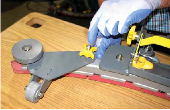
9. Position the squeegee assembly bracket near the squeegee carriage and align the squeegee carriage pins into the squeegee assembly bracket.
