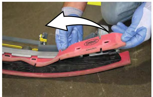
7. Rotate the rear blades to a new wiping edge and reinstall blades. Make sure to align the slots in the blades with retainer tabs.
