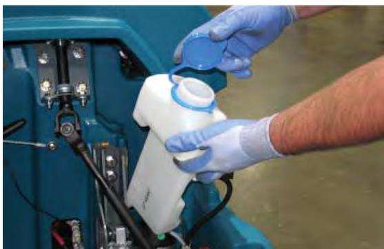
The automatic battery watering indicator will also alert user to add distilled water when tank is empty. See CONTROL PANEL OPERATION for further details.
