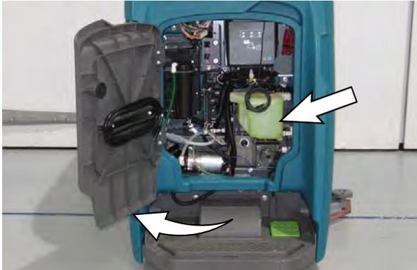
2. Remove the Severe Environment tank from the machine and set it on the floor.
