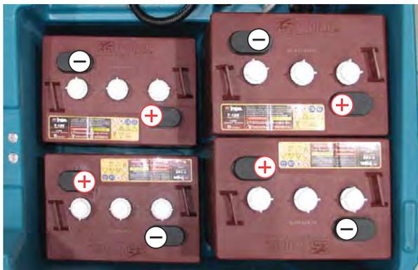
3. Using the supplied battery post boots, connect the cables to battery posts, RED TO POSITIVE (+) & BLACK TO NEGATIVE (-). Tighten cable connections to batteries per battery manufacturer specifications.
