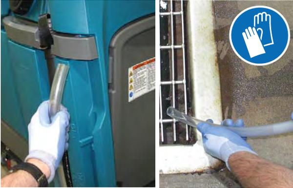
3. Rinse solution tank with clean water. Firmly reconnect the hose to the solution tank after rinsing / draining tank.
