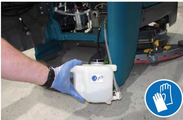
**NOTE:** Remove the Severe Environment tank from the machine before filling the tank with detergent to prevent damaging electronic components.
