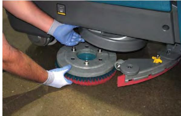
4. **Machines equipped with magnetic brush hubs:** Push the new brush or pad driver under the scrub head and lift the brush or pad driver until the magnet secures the brush or pad to the drive hub.
