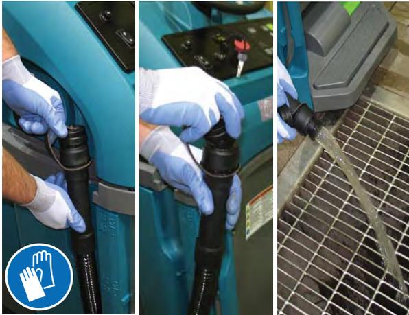
*NOTE: When using a bucket to drain the machine, do not use the same bucket to fill the solution tank.*
