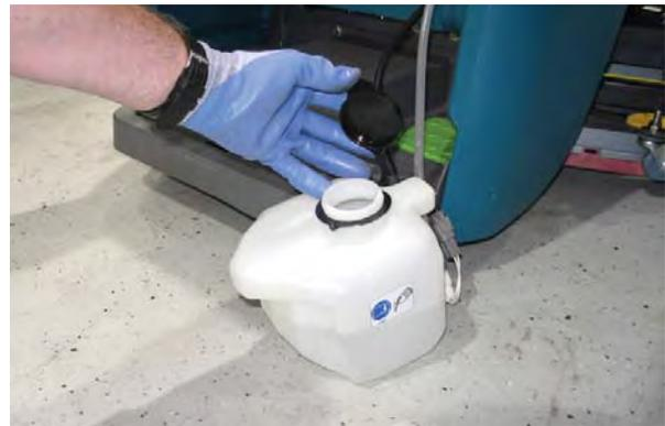
10. Automatic battery watering option - Refill tank with distilled water. Replace cap.
