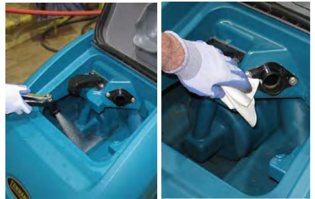
**FOR SAFETY: When servicing machine, do not power spray or hose off machine. Electrical malfunction may occur. Use damp cloth.**
