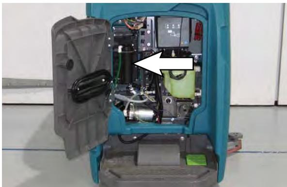
3. Disconnect the two hose connectors from the top of the cartridge by pressing the gray collars inward and pulling the connectors outward. Lift cartridge to remove.
