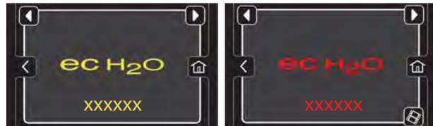
*NOTE: If a fault occurs to the ec-H2O system, the machine may automatically turn off the ec-H2O system and convert over to conventional scrubbing. The service indicator button will continue to flash until the ec-H2O fault is serviced.*
