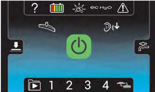
**Supervisor Mode** - Capable of machine operation with full use of all controls, along with configuring permissions and restrictions for the operator mode and login capability. The supervisor mode home screen provides access to the machine settings button and to the maximum scrub speed button.
