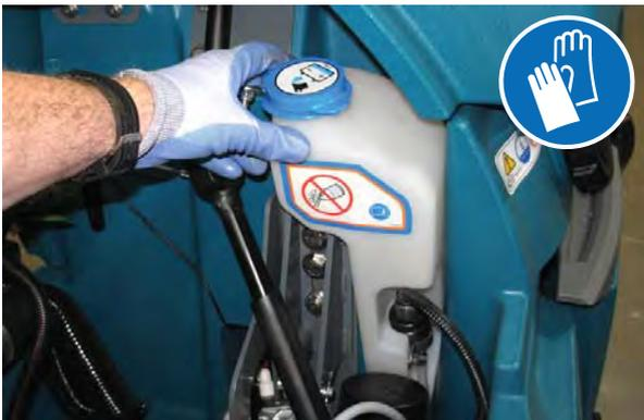
3. Remove the blue cap from the automatic battery watering tank.
