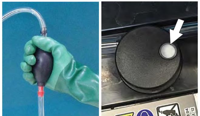
6. After adding water, store the hand pump hose inside the machine's battery compartment for future use.
