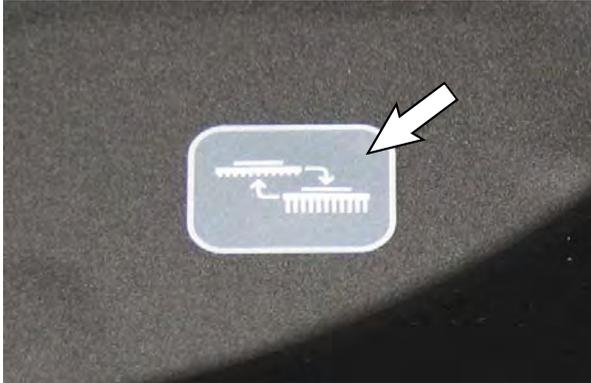
**Machines with magnetic brushes:** Press the brush change button to release the brush(es) from the scrub head. The scrub head will completely raise to disengage the brush(es) from the scrub head, and then partially lower to allow the brush(es) to be removed from under the scrub head. Reinstall brush(es) with scrub head in partially lowered position.
