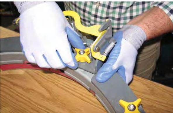
9. Position the squeegee assembly bracket near the squeegee carriage and align the squeegee carriage pins into the squeegee assembly bracket.
