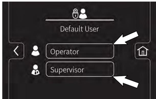
7. Select a pre-assigned user profile. In this example, operator profile "JOHN" is selected. Turn the key off to apply the setting.
