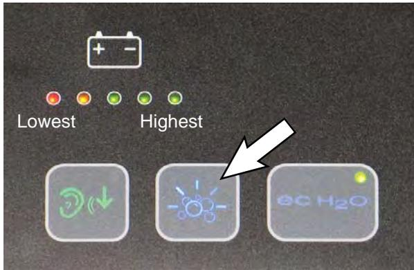
*NOTE: The maximum scrub speed setting can only be adjusted in supervisor control lockout modes 2 and 3.*
