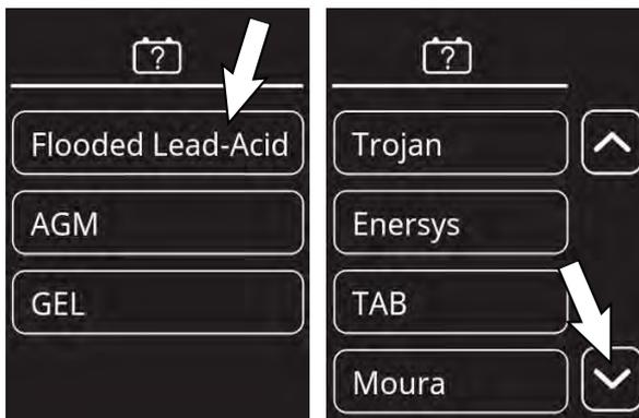
*NOTE: The battery charger profile and battery discharge indicator will automatically reprogram when battery type is selected.*
