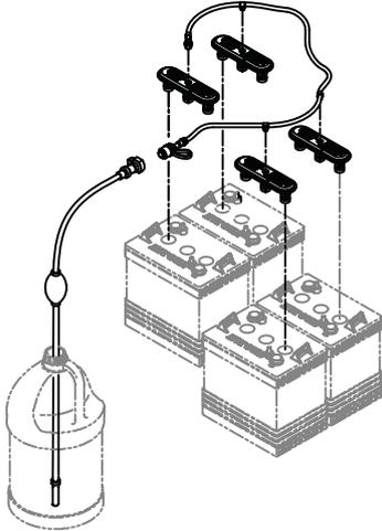
The optional HydroLink battery watering system provides a safe and easy way to maintain the proper electrolyte levels in your batteries. It is designed exclusively for Trojan flooded (wet) lead-acid batteries.
