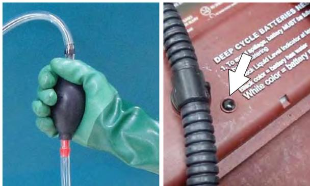
6. After adding water, replace the dust cap on the battery fill hose and store the hand pump hose inside the machine's battery compartment for future use.
