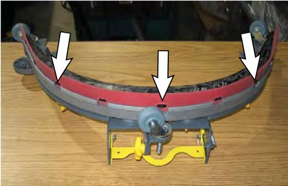
8. Squeeze the squeegee frame and blade retainer together and re-tighten the four knobs.
