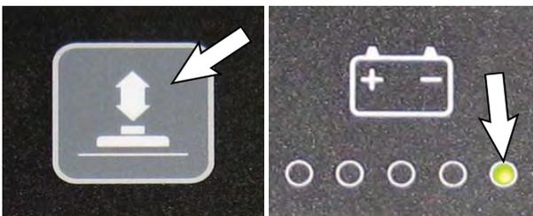
3. To select or change a supervisor control mode, press and hold the specific zone control button until the LED blinks three times. For lockout mode 3, press and hold zone control buttons 1 and 2 at same time. After selection is made, the LED will turn solid to indicate new mode.
