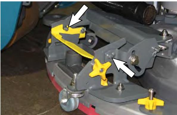
5. **Machines with 20 in. (500 mm) scrub heads only:** Be sure both squeegee tabs are positioned above the scrub head skirt.
