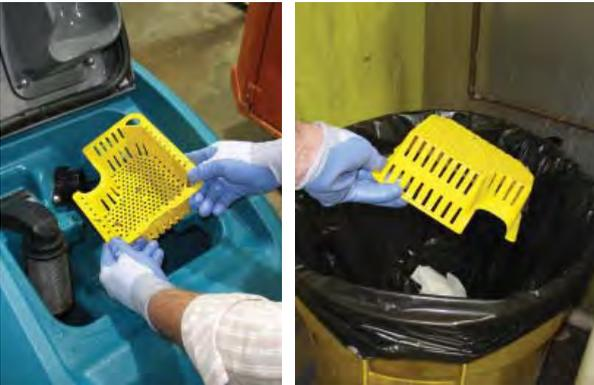
7. Remove and clean the float shut-off screen.
