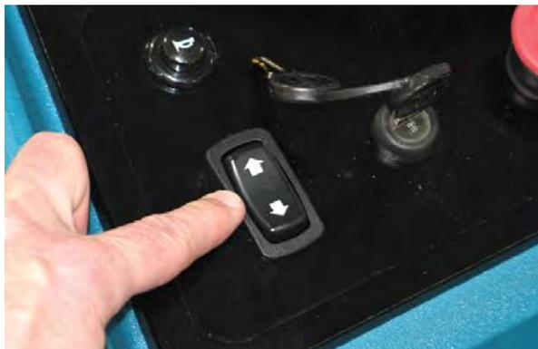
*NOTE: If forward / reverse switch lights are flashing rapidly, be sure right foot is not pressing the green go pedal. The machine will not accept input from the forward / reverse switch if the lights are rapidly flashing.*
