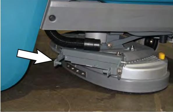
3. Align the squeegee carriage pins into the squeegee assembly bracket.
