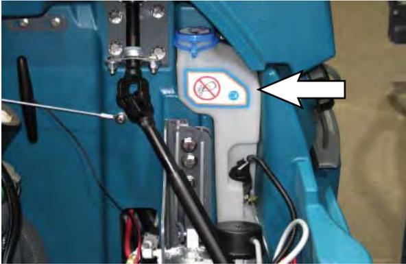
2. Reposition the automatic battery watering tank so that it can be easily filled.
