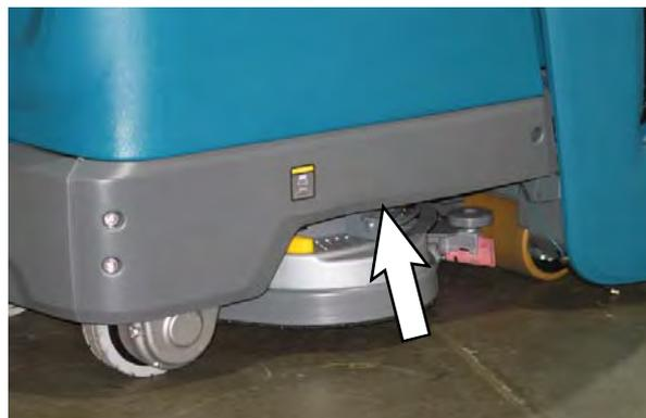
4. Position a floor jack under the tie down / jack point and arrange all hoses / cables so they are not crushed when the machine is jacked up off the floor.
