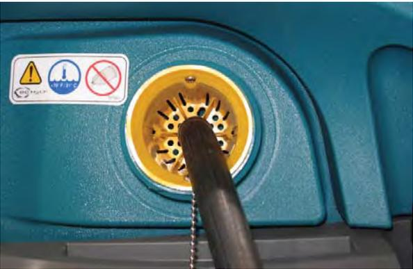
3. Fill the solution tank with water until level reaches the 53 L (14 G) mark on the solution tank indicator.
