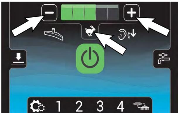
4. Press the (+) button to increase the maximum scrub speed. Press the (-) button to decrease the maximum scrub speed.
