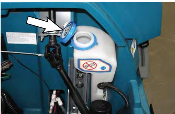
4. Pour distilled water into tank. To avoid getting water on sensitive components, use a funnel to fill automatic battery watering tank.
