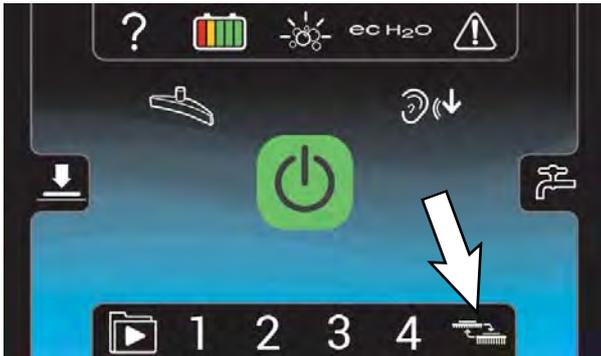
*NOTE: Remain standing on the operator presence pedal until the scrub head has moved through the entire range of motion and has stopped moving. Process will be paused if the operator presence pedal is released. Step back onto the operator presence pedal and press brush change button again to continue the process. Turn key switch to OFF position to abort process.*
