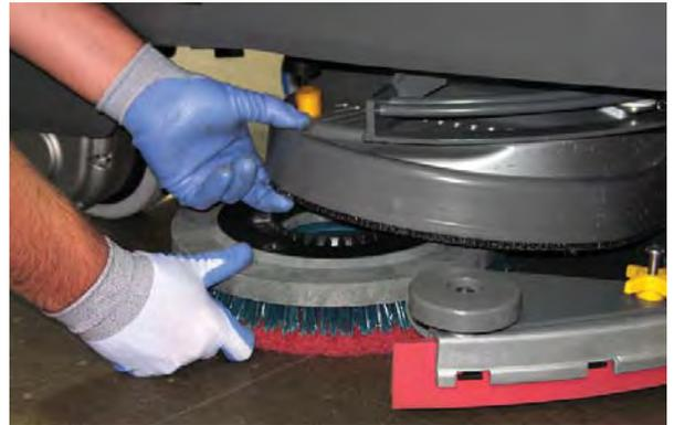
**Machines with 3-lug brush hubs:** Position the three lugs into the motor hub slots and give the pad driver / brush a quick counter-clockwise turn to engage hub.
