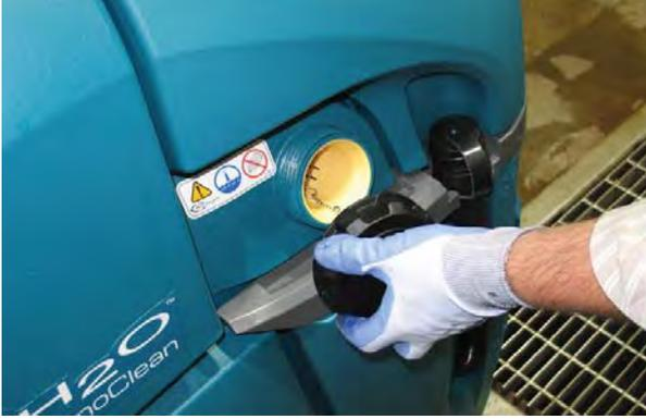
2. Insert the fill hose into the yellow strainer and ensure the hose is held securely into place in the strainer.
