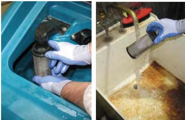
8. Drain and rinse out the solution tank.
