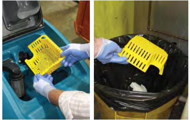
Rinse out the recovery tank with clean water and wipe clean of any soil residue.
