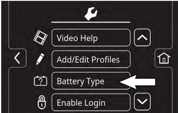
4. Select battery type and brand installed in machine. See battery label to determine type and brand. Press the up and down arrows to scroll through battery selection.
