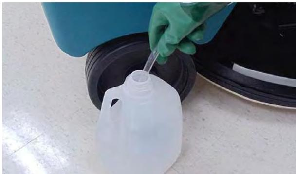
5. Squeeze the bulb on the hand pump hose until firm. The level indicators will turn black when full.
