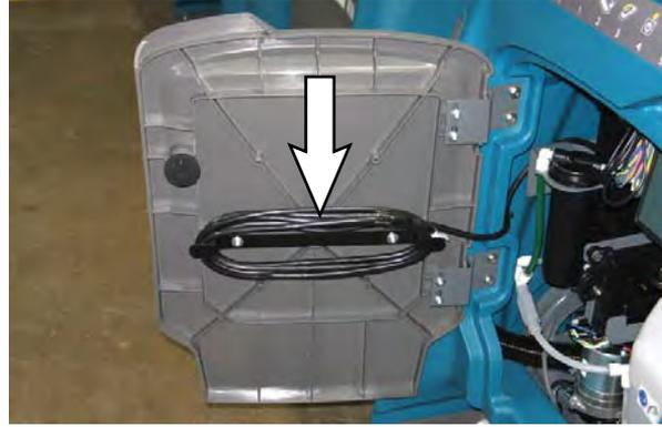
For models equipped with off-board chargers, first connect the charger's DC cord into the machine's battery charge receptacle then plug the AC power supply cord into a properly grounded wall outlet. Refer to the off-board battery charger's owner manual for operating instructions. Do not close the recovery tank on the charger cables when charging with an off-board charger.
