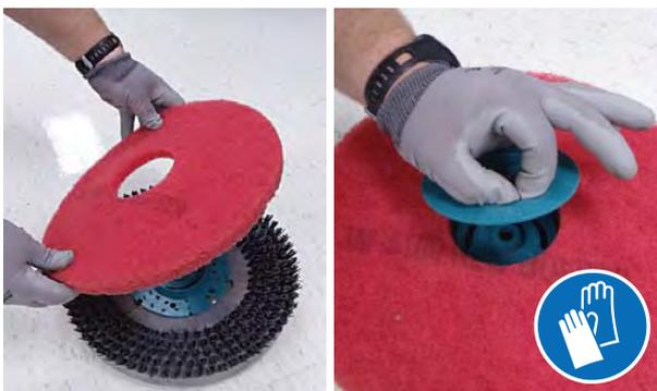
3. **Machines with magnetic brushes or pad drivers:** Position the brush under the scrub head and lift the brush up onto the scrub head until the magnet in the scrub head secures the brush.
