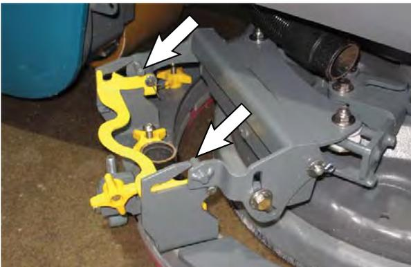
10. Slide the squeegee assembly onto the squeegee carriage until both squeegee carriage pins are secured in the bracket.
