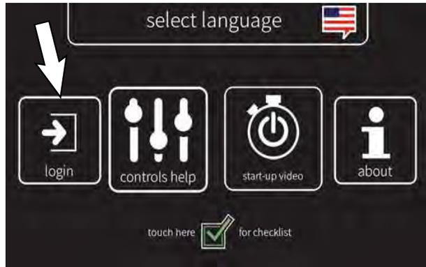
3. First time use - Enter the factory-assigned supervisor mode login code "1234" then press the green enter button.
