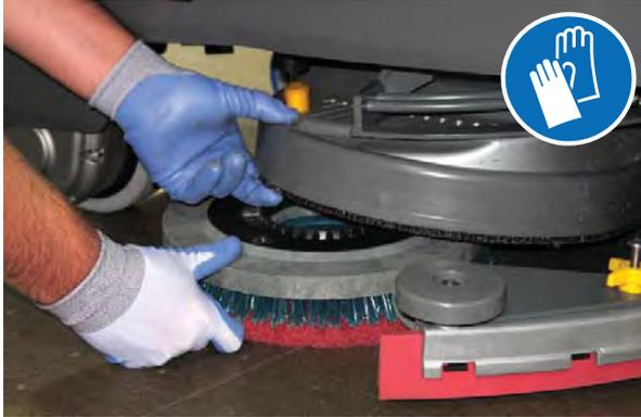
**Machines equipped with 3-lug brush hubs:** To remove the brush or pad driver, grip the disk and give it a quick turn.
