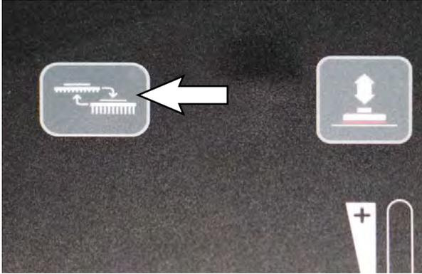
*NOTE: Remain standing on the operator presence pedal until the scrub head has moved through the entire range of motion. Process will be paused if the operating presence pedal is released. Step back onto the operator presence pedal and press the brush change button again to continue the process. Turn key switch to OFF position to abort process.*
