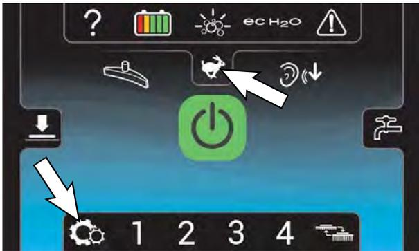
**Operator Mode home screen** restricts access to the machine settings button and maximum scrub speed button.
