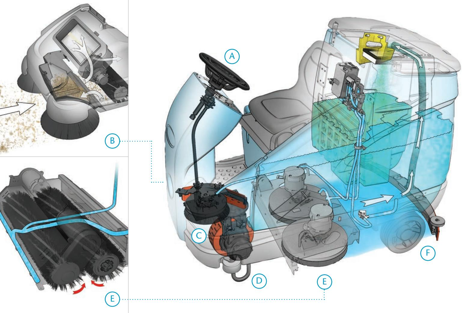
**A** Reduce operator fatigue and effort with a flex-shaft steering system that provides smooth and easy steering.
