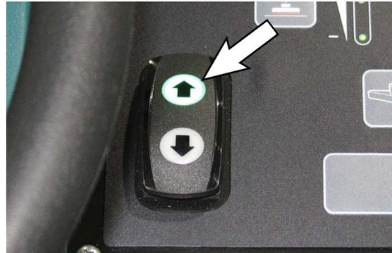
*NOTE: The squeegee automatically raises when the machine is driven backwards. This prevents damaging the squeegee. When the machine is placed in reverse, the vacuum fan will shut off after a short delay.*
