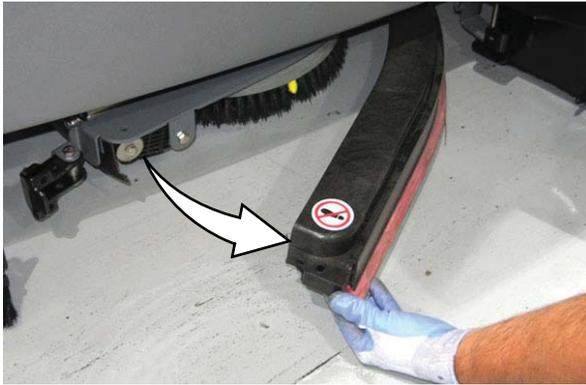
6. Press the spring clip together with the thumb and index finger. The brush/pad driver will drop off the drive hub. Remove the brush from under the machine.
