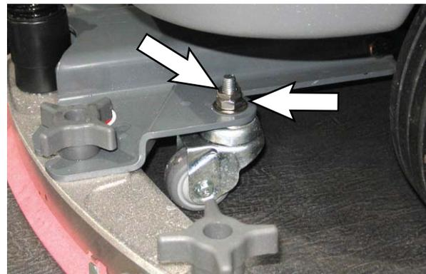
5. Drive the machine forward again to recheck the squeegee blade deflection after adjustments are made.
