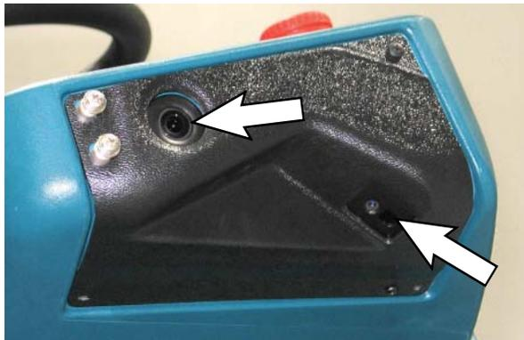
**UPPER AND LOWER LIDAR SENSORS**
