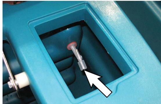
7. Replace the recovery tank drain hose cap and mount the drain hose back onto the mounting clip after the tank is drained.
