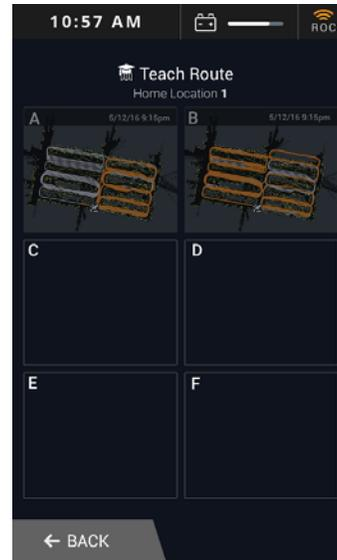
*NOTE: In the above screen routes A and B are already being used for robotic routes. Routes C, D, E, and F are available for new routes.*
