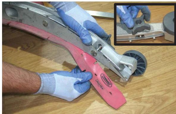
8. Install the new front squeegee blade or rotate the existing blade to the new edge. Be sure the holes in the front squeegee blade are hooked onto the tabs on the front blade clamp.
