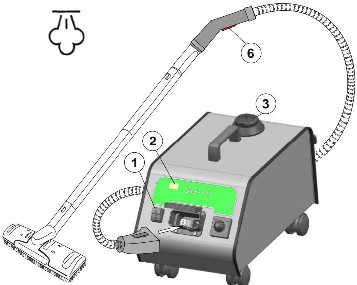
When the machine is ready, to release steam through the handle of the flexible, press the lever button (6). Now use the brush or accessory in the surfaces to be cleaned.
